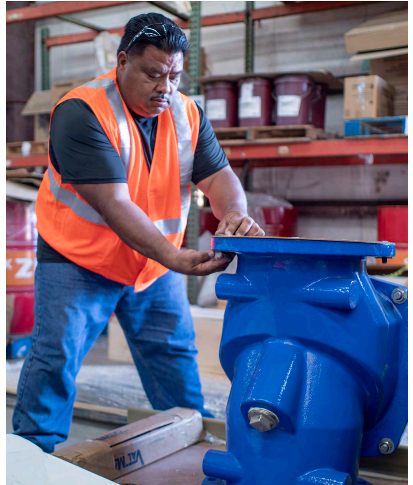
Heavy Equipment Mechanic Leader Roy Chargualaf inspects a check valve in the warehouse in preparation for a valve installation.
