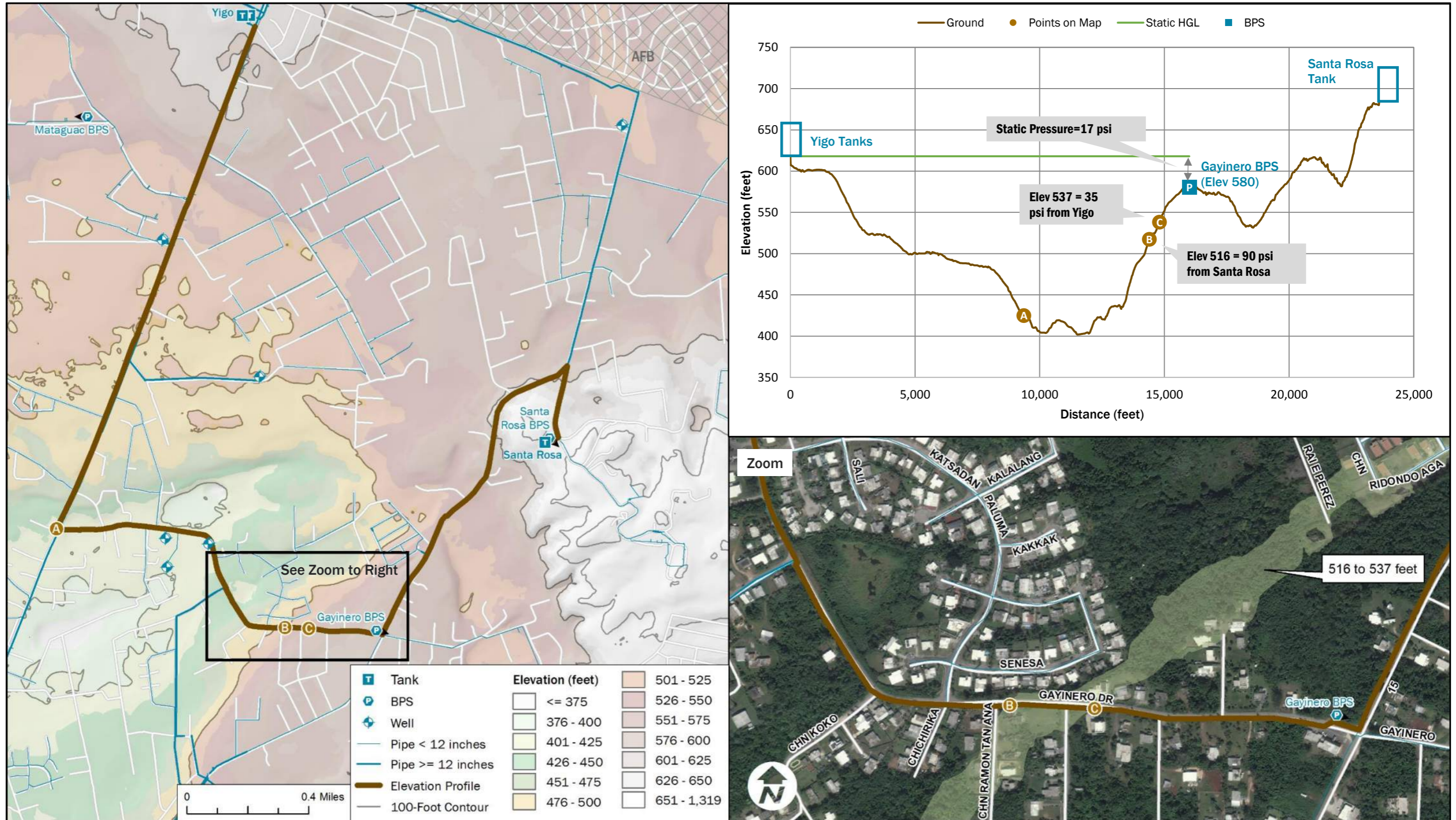
Figure 7-1. Profile of Piping from Yigo Tanks to Gayinero to Santa Rosa Tank
