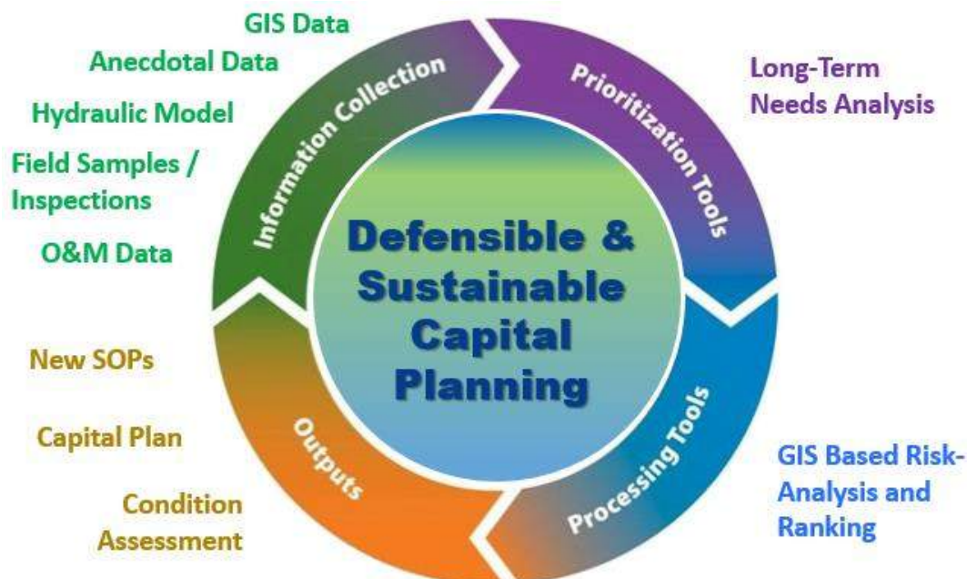
Figure 8-5. Diagram of the Approach to Ranking Water Piping
